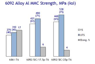
AL MMCS ARE CONVENTIONALLY HEAT-TREATED. THE PRESENCE OF SIC PARTICLES IN THE ALUMINUM MATRIX ACCELERATES precipitation aging kinetics. Peak strength (T6) through artificial aging is achieved in approximately 8 hours, while natural aging (T4) can achieve peak strength after 96 hours.
