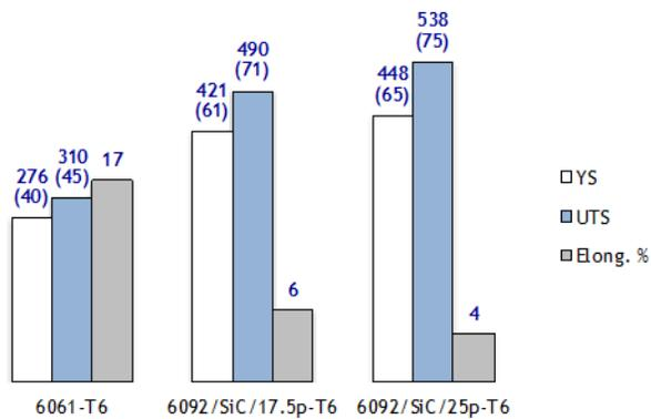
**AL MMCs ARE CONVENTIONALLY HEAT-TREATED. THE PRESENCE OF SiC PARTICLES IN THE ALUMINUM MATRIX ACCELERATES** precipitation aging kinetics. Peak strength (T6) through artificial aging is achieved in approximately 8 hours, while natural aging (T4) can achieve peak strength after 96 hours.
